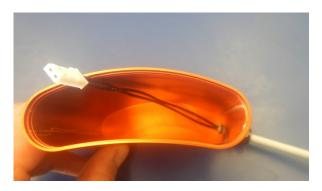
Firstly make sure that the end of the grey cable arrives in the battery case like this (not more!) and tighten well the black feedthrough.
