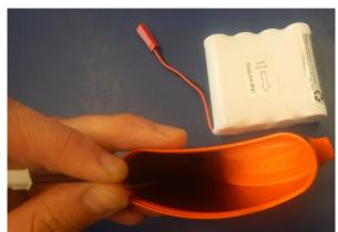
Now press the black cables right to the wall and slip the battery into the battery case as indicated on the small sticker on the battery (upside down!)
